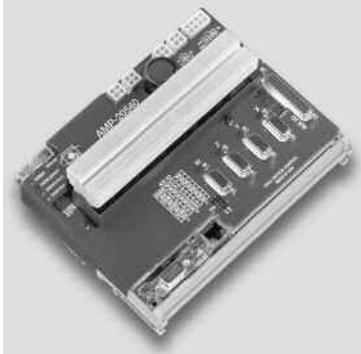
AMP-20540 Interconnect with 4-axis 500 W servo drives
