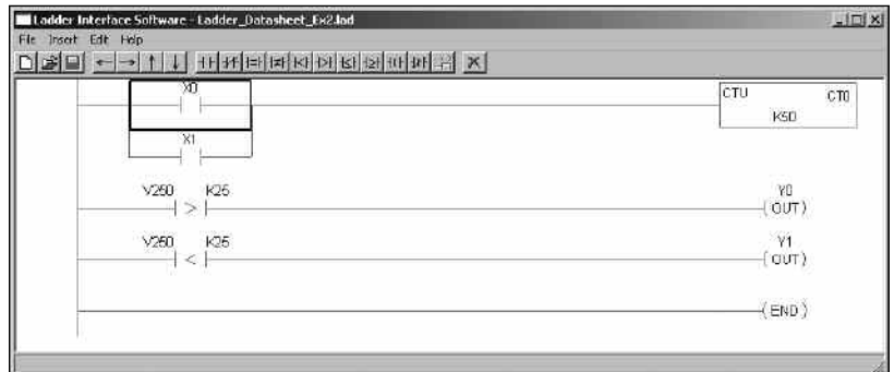
Up-Counter (CTU) and comparative logic example
