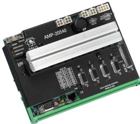
Figure 3. DMC-2133-DC24-DIN with attached AMP-20540
