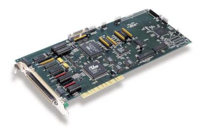
Galil's new enhanced firmware is designed for its PCI (DMC-18x0 shown) and Ethernet motion controllers.
