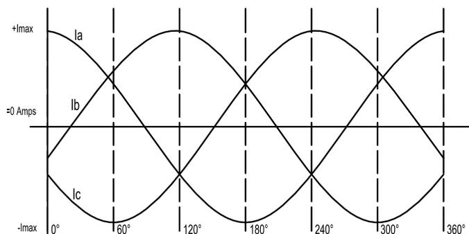
Figure 3: Sinusoidal current output based on electrical angle
