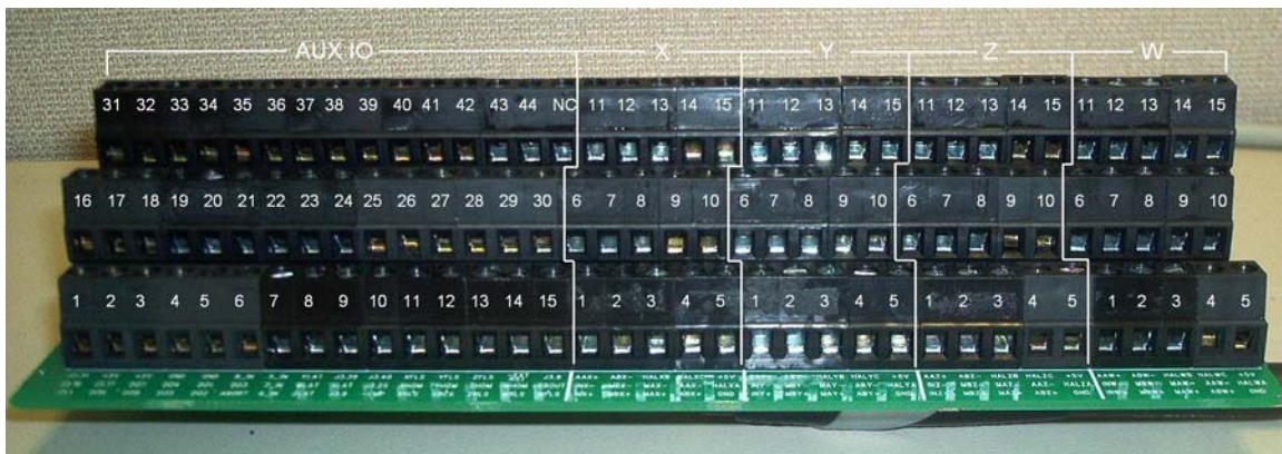
Fig. 1– Image of ICM-19540 screw terminals with labeling
